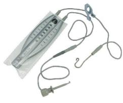
the distance from the tip of the endodontic file to the foramen. The Mark VII allows dental professionals to know the depth of the canal by showing when they are 2.0 mm, 1.5 mm, 1.0 mm, 0.5 mm, 0.25 mm away from, and then the apex has been reached.
